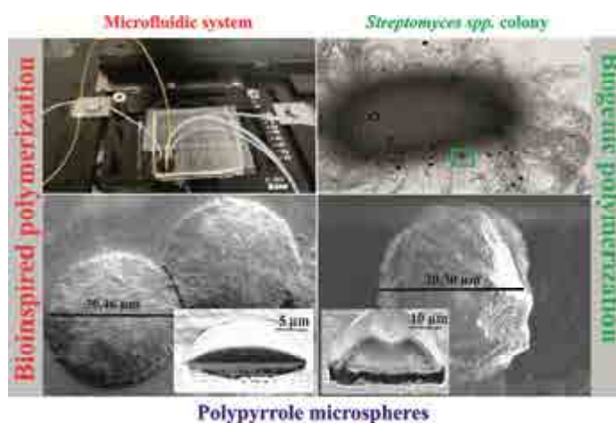
Fig. 1. Different methods of polypyrrole synthesis. (Left, above) Microfluidic system for microemulsion polymerization and (left, below) the microspheres obtained by this method. (Right above and below) Streptomyces spp. colony with polypyrrole microspheres. Insets: the cross sections of microspheres obtained by different methods.
