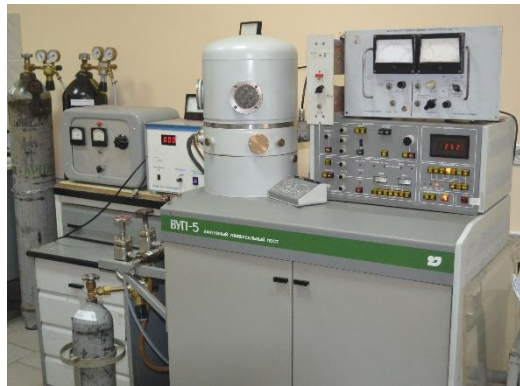
Equipment for deposition of thin films and electrodes. (a) VUP-5; (b) SC7620 and CA7625.
