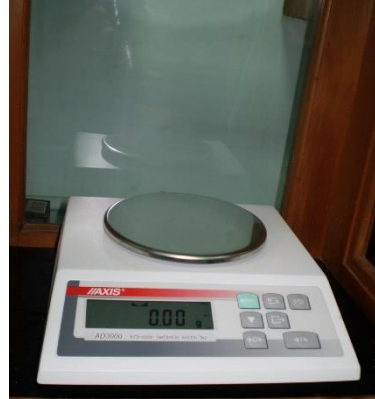
Analytical scales for weighing the initial reagents and equipment for synthesis.
