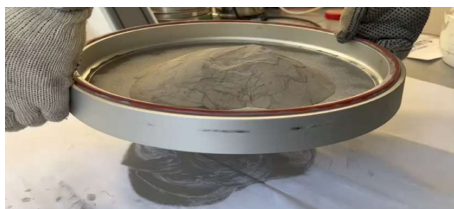
Figure 1) Developed ultrasonic sieve for material preparation
