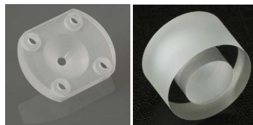
Fig. 12. The nozzle (35 mm-diameter, 12 mm-height) with a 2 mm-length channel with the output diameter of 100 \mu\text{m} , machined in fused silica combining the rear-side laser processing and laser-assisted selective etching technology, and optical element with laser cut hole.
