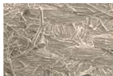
Fig. 3. SEM-image of a sample with an optimal coating deposit.
