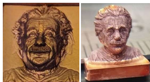
Fig. 13. 3D Albert Einstein's face profile milled by a picosecond laser in bulk copper, dimensions 10×10×2 \text{mm}^3 .
