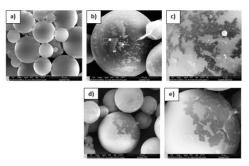
Fig. 1. SEM morphologic analysis of microcapsules MPCM32D: (a) unmodified, magnification 5000x; (b, c) with 5wt.% MWCNTs shell-modified, magnification 5000x and 10000x; (d, e) with 5wt.% PEDOT: PSS shell-modified, magnification 5000x and 10000x.
