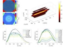
Fig. 2. Distribution of the retardance  $\tau$  and the slow axis  $\theta$  in the PBP element manufactured by Altechna R&D. (Top) The 3D intensity distribution in the optical needle created by the combination of the PBP element, the linear polarizer and the axicon. (Bottom) Distortions in the optical needle caused by the azimuthal misalignment between the polarizer and the PBP element for various values of the mismatch apple  $\theta$
