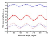
Fig. 7. Azimuthal angle dependences of THz emission from two samples: VS001 (blue) and VS002 (red). The spectra were measured in the transmission geometry:  $\theta$ =30° (full lines) and  $\theta$ =0° (dashed lines).
