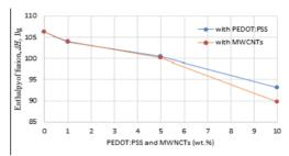
Fig. 2. The influence of shell modifiers PEDOT: PSS and MWCNTs on fusion enthalpy of paraffin PCM microcapsules.
