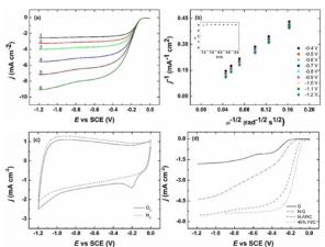
Fig. 3. RDE voltammetry curves for oxygen reduction on GC electrodes modified with different catalyst materials in  $O_2$ -saturated 0.1 M KOH for v = 10 mV  $s^{-1}$  and  $\omega$  = 1900 rpm.
