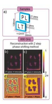
Fig. 1. Two 2D objects reconstruction at 600 GHz frequency using the phase shifting technique and Angular Spectrum of Plane Waves propagation method.
