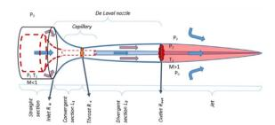
Fig. 17. De Laval nozzle geometry components.
