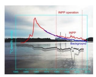
Fig. 6. Measured and calculated values of <sup>14</sup>C specific activity in the alkali-soluble and alkali-insoluble sediment fractions.
