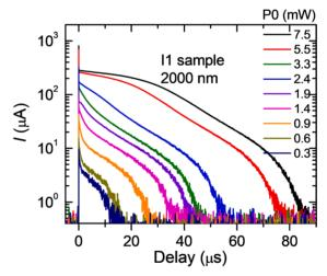
Fig. 10. Temporal response (photocurrent relaxation curves) of GeSn IR photodiodes (I1 sample) under 0.5 V reverse bias using different laser power at wavelength of 2000 nm. With the excitation increase, the response of the photodiode becomes slower due to the screening of charge separation potential by injected carriers.
