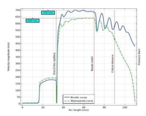
Fig. 18. Comparison of the velocity of Bicubic and Witoszynski curve
