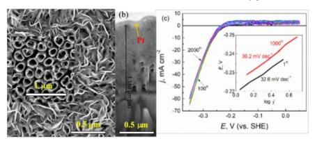
Fig. 5. (a) Top-side and (b) cross-sectional SEM images of hybrid MoS $_2$ /cyst film whereas (c) depicts the CV plots in 0.5 M H $_2$ SO $_4$  solution up to 2000 potential scans. Insets: in (a) support SEM view, in (c) Tafel slope for indicated scan.
