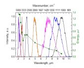
Fig. 8. The LGS OPA idler wave output spectra and pulse energies in the wavelength tuning range of 2 - 9.6  $\mu$ m.
