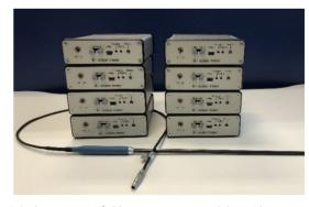
Fig. 8. B-Scalar magnetic field measurement modules with semiflexible probe. The project was project supported by MITA (Project Nr. 01.2.2-MITA-K-702-06-0012).
