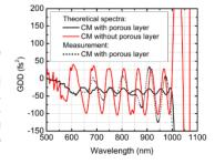
be approximately 1 % due to the changes in humidity. In addition, GDD oscillations of the coatings exhibited low sensitivity to deposition errors of porous layer and humidity in the surrounding environment. Presented results are essential for applications in femtosecond lasers, where GDD oscillations are limiting their performance.
