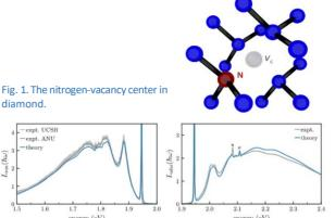
Fig. 2. Calculated (left) luminescence and (right) absorption lineshapes at nitrogen-vacancy centers in diamond (blue curves), compared to experimental ones (gray curves).
