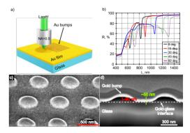
Fig. 2. (a) Illustration of Au bumps formation in a thin gold film using direct laser writing technique; (b) reflectance spectra of microbumps array with period 700 nm in 50 nm thick gold film at a different angle of incidence for *p*-polarized light; (c) SEM micrograph of fabricated gold bumps array in a thin gold film (50 nm); (d) cross-section of gold bumps.
