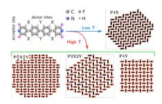
Fig. 4. (Top, left) BDFPBP molecule and (top, right and bottom) four self-assembled structures obtained by MC modeling. Black rectangle represents the molecule with differently damaged (red boxes) donor sites.
