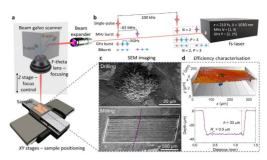
Fig. 1. Investigation of ultrafast laser burst-mode processing influence on ablation efficiency. (a) Principal scheme of laser processing setup. (b) Illustration of four possible laser working regimes: single-pulse, MHz burst, GHz burst, and biburst. (c) SEM images illustrate laser drilling and milling of copper samples and (d) corresponding graphs for efficiency evaluation.
