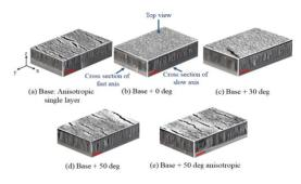
Fig. 14. The 3D representation of SEM images combination of (a) single layer with 250 nm thickness, deposited at an angle of  $70^{\circ}$  and 2-layers structures with the second layer deposited at (b) 0, (c) 30°, (d) 50° and (e) 50° -anisotropic case. The red bar is set at 250 nm.
