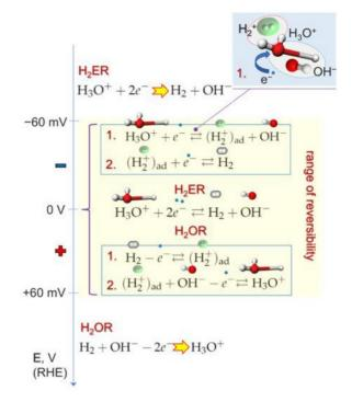
Fig. 4. Hydrogen evolution/oxidation reactions  $H_2ER/H_2OR$  in aqueous solutions. Inset: schematics of  $H_2^+$  formation using pictorials of chemical structures of the participating species.
