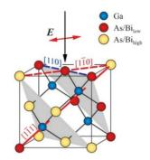
Fig. 3. (Top) Atomic structure of GaAsBi, showing CuPt-type ordering of Bi atoms on every second (111) plane. (Bottom) Photo-modulated transmission spectra of GaAsBi indicating in-plane polarization direction dependence and valence band splitting.
