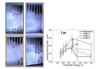
Fig. 16. The ER dependence on the pulse energy for vertical structures etched from the top surface in 10M KOH for 2 hours. The modifications were inscribed through the whole sample thickness. Dark areas from the top and bottom show the etched material. Laser pulse duration is 1 ps. The z-step distance was set to 5  $\mu m$ . The colour border of the microscope pictures corresponds to the curve colour on the graphs. The error bar shows the standard deviation from the averaged value.
