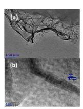
Fig. 2. (a), (b) TEM images of wood-derived N-doped carbon.
