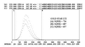
Fig. 1. Effect of quenching for the LSC cocktail (GSLT) at the sample-to-cocktail ratio of 10:10 mL. The spectra [B] and [C] are measured with added 20 and 40  $\mu l$  of quenching agent, respectively. The SQP(E)=724 refers to the typical sample prepared with the GSLT cocktail.
