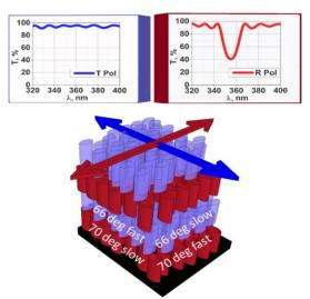
Fig. 15. The principal scheme of cross-sections of polariser for normal incidence angle, based on multi-layer coating consisting of anisotropic layers with perpendicularly aligned optical axes.
