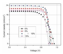
Fig. 6. Current voltage characteristics of perovskite SCs with different cesium concentrations.
