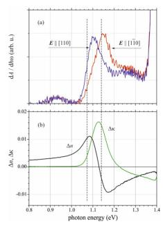
Fig. 11. (a) Optical density differential spectra and (b) the spectra of birefringence  $\Delta n = n_{[110]} - n_{[1\bar{1}0]}$  and linear dichroism  $\Delta \kappa = \kappa_{[110]} - \kappa_{[1\bar{1}0]}$  for the GaAs<sub>1-x</sub>Bi<sub>x</sub> (x=0.042) sample. Vertical dashed lines indicate spectral positions of the optical features observed in photo-modulated transmittance / reflectance spectra.
