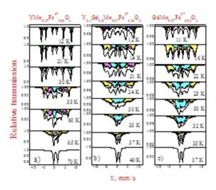
Fig. 2. (a) Mössbauer spectra of YMn $_{0.97}$ Fe $_{0.03}$ O $_3$ , (b) Y $_{0.4}$ Gd $_{0.6}$ Mn $_{0.97}$ Fe $_{0.03}$ O $_3$  and (c) GdMn $_{0.97}$ Fe $_{0.03}$ O $_3$  (c) at indicated temperatures.
