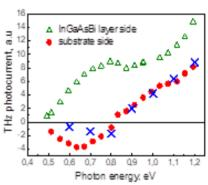
Fig. 4. The THz excitation spectra measured after InAsGaBi/InP structure excitation by femtosecond optical pulses from the layer and from the substrate side. Blue crosses are the results of the Monte Carlo simulation.
