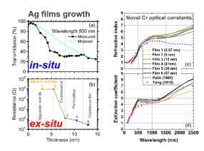
Fig. 4. (a) Transmittance and (b) resistivity versus thickness of silver films. (c) Refractive index and (d) extinction coefficient of ultrathin chromium films.
