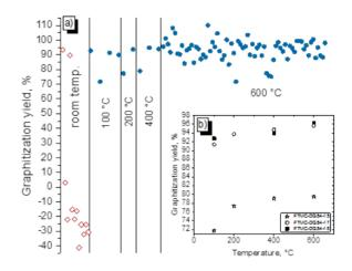
Fig. 4. (a) Graphitization yield of samples with a sulfur trap at temperature above  $100^{\circ}$ C (blue circles) and room temperature (red diamonds). (Inset) Graphitization yield of the three cremated bone samples at different temperatures.
