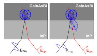
Fig. 5. The momenta of electrons excited from the heavy hole subband in the narrow bandgap part of heterostructure by linearly polarized femtosecond light pulse. (Left) The electron excess energy lower than the conduction band offset; (right) higher than the offset.
