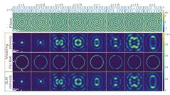
Fig. 3. Intensity patterns of non-diffracting beams as a function of the spatial displacement between two halves of axicon masks. The displacement p is given in steps of quarter period. The phase period  $r_0$  = 80  $\mu$ m and the Bessel beam cone half-angle  $\theta_c$  = 0.74 $^{\circ}$ . Bottom rows depict intensity distribution of experimentally generated beams.
