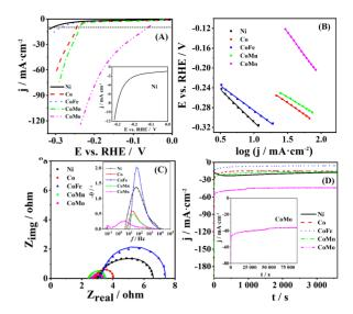
Fig. 1. (A) HER polarization curves (iR-corrected) of five studied coatings at 5 mVs- $^1$  with (B) corresponding Tafel plots. (C) Nyquist plots at -0.33 V (amplitude of 5 mV in the 100 kHz–0.1 Hz range) with the corresponding Bode plots in the inset. (D) Chronoamperometric curves at -0.24 V for 1 h with the chronoamperometric curve of CoMo at the same potential for 24 h (inset). All measurements were performed in 1 M KOH.
