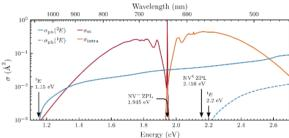
Fig. 3. Calculated photoionization cross section from the excited state 3E (blue curve), cross section for stimulated emission (dark red curve), and cross section for absorption (orange curve) for nitrogenvacancy centers in diamond.
