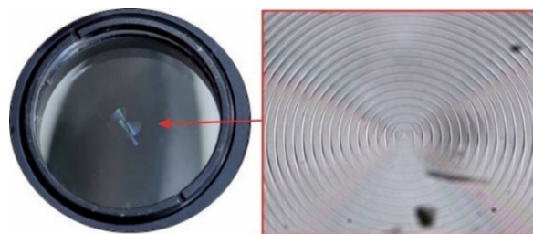
Demonstrator of the fraxicon recorded in the volume of UVFS glass by laser writing technology.
