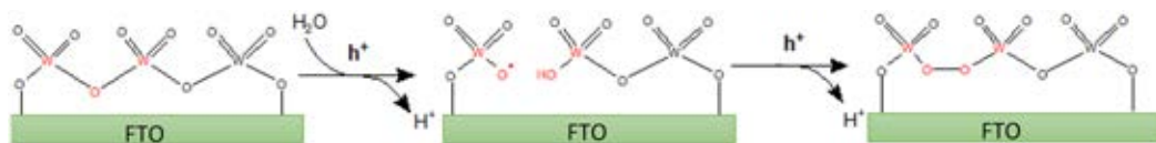
Fig. 11 Mechanism of hole-induced formation of peroxo species on the surface of WO_3 film
