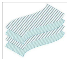
Fig. 1. Structure of one layer UHMWPE laminate (0/90/0/90° ply) [1].
