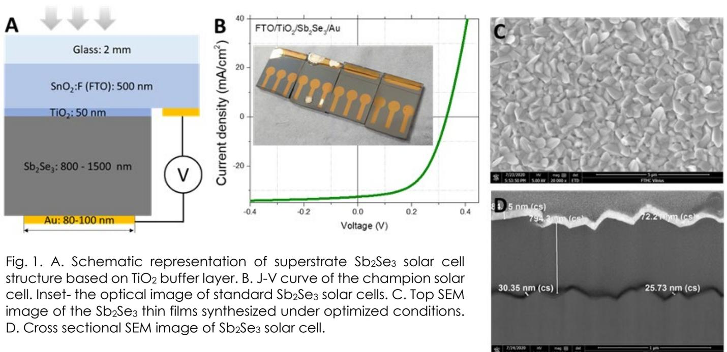
Fig. 1. A. Schematic representation of superstrate  $\text{Sb}_2\text{Se}_3$  solar cell structure based on  $\text{TiO}_2$  buffer layer. B. J-V curve of the champion solar cell. Inset- the optical image of standard  $\text{Sb}_2\text{Se}_3$  solar cells. C. Top SEM image of the  $\text{Sb}_2\text{Se}_3$  thin films synthesized under optimized conditions. D. Cross sectional SEM image of  $\text{Sb}_2\text{Se}_3$  solar cell.
