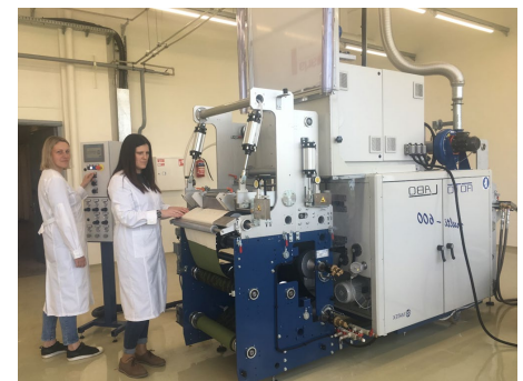
Fig. 1. Rotolabo Multi 600 ("Matex"), pilot continuous coating and laminating machine.
