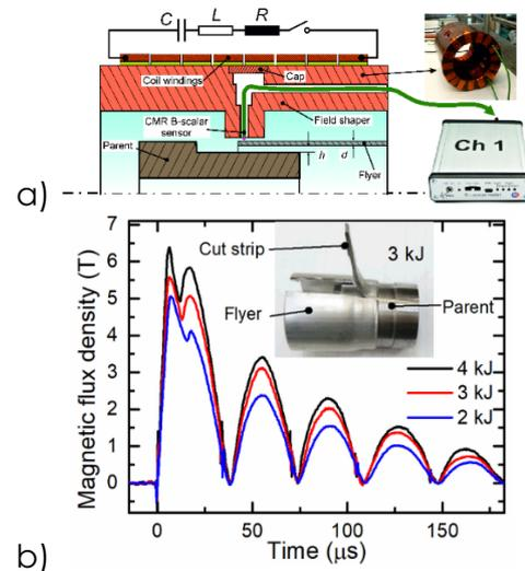
Fig. 1. Setup for magnetic pulse welding of tubes to cylinders with installed CMR-B-scalar probe for magnetic field measurement (a). Magnetic field between the field shaper and aluminum flyer tube at different charging energies (b). The inset presents a picture of the tested specimen after MPW.
