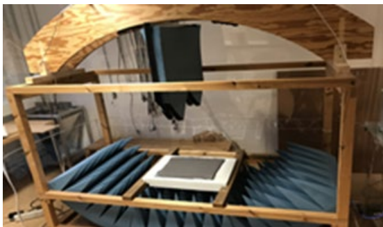
Figure 1. Microwave reflection measurements at FOI: photo of the NRL arch setup
